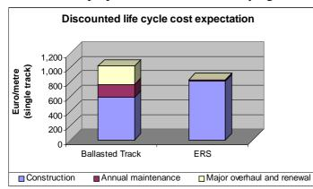
necessary *preparatory work* differ for different subgrades. Although construction costs of the railway track were about 40% higher than ballasted track, the total discounted life cycle costs were calculated to be 20% less than those of the ballasted track used in the Netherlands, which are about 2300 guilders per metre (figure 6). A rail renewal was not needed in the period considered and this means that only some annual maintenance is foreseen. Costs of inspection and
