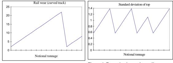
Figure 3 Example change in quality (rail wear)
